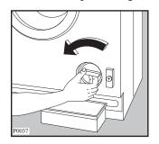
Unscrew and remove the filter.
